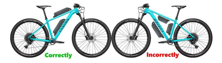
Installing the battery upside down will damage it soon after you start using it.
