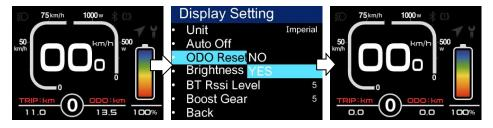
On the main interface, press and hold the "+" and "-" keys at the same time to achieve zero TRIP and AVG, as shown in the following figure:
