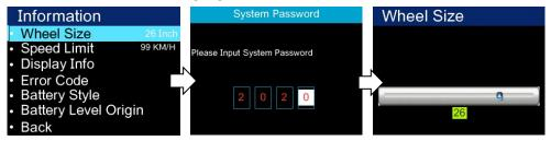
2 Speed Limit Information - Go to the Speed Limit menu(Need to enter the password 2020, which cannot be modified). When the unit is kilometers (metric), the default speed limit is 99 km/h, 0~99km/h optional.
