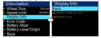
Error Code – Go to the Error Code menu, "E-CODE 0" refers to the last error message, and "E-CODE 9" refers to the tenth error message. Records can have up to 10. Press "+" or "-" to toggle. Error code "00" indicates no error. For the meaning of the other codes, see the error code definition table. As shown in the following figure:
